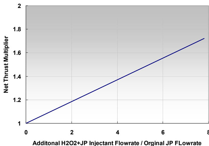
Figure 18. Rocket augmentation impact on the engine thrust, Ref. 10.
