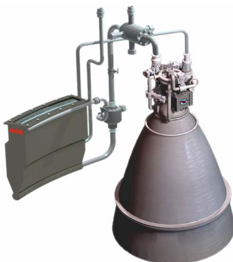
Figure 15. AspiRE cycle based on RL50 engine, Ref.8.
