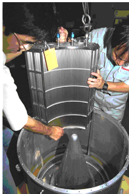
Figure 4: Assembly of the quarter of the BARABAN-type precooler. (Picture acquired from the ISAS website http://atrex.isas.ac.jp/ ).
